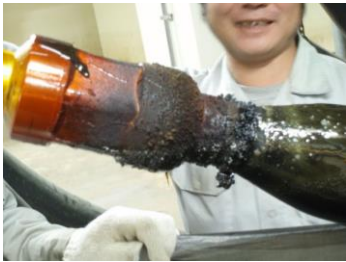
Figure 19 PDs caused by poor installed cable termination
